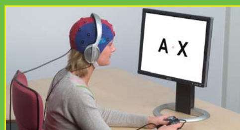
Figure 4: eevoke allows you to present visual and auditory stimuli at the same time.
